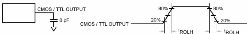
Figure 9. Receiver LVTTTL/CMOS Output Load and Transition Times
